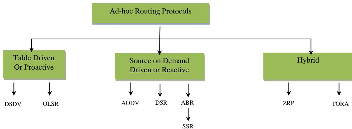
Figure 1: Classification of MANETs Routing Protocols.
