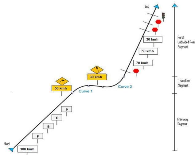
Fig. 2 Road geometry for driving simulator scenarios
