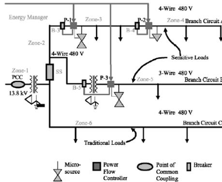
The CERTS Micro Grid has presents unique electrical analysis challenges such as contain three phase, single phase and variety of sources interconnected by power electronic devices employing different control approaches. The modeling approach enables analysis of a variety of issue such as prediction and evaluation of imbalance, asymmetries, generation-load control and dynamic voltage.
