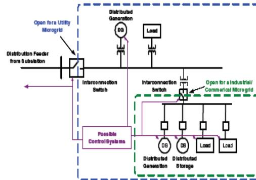
There are many potential benefits to customers from the use of microgrids including improving reliability by providing power to the islanded portion of the electric power system (EPS) during a utility outage and resolving power-quality issues by reducing total harmonic distortion at the loads.
