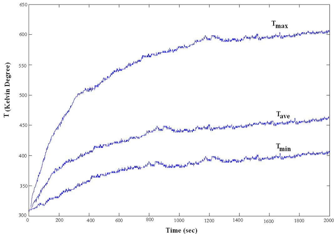
Figure 3. Maximum, average and minimum temperature variation of the heated plate versus time to achieve steady state condition ( $h=3.5$  cm,  $Q = 2000$  watt)
