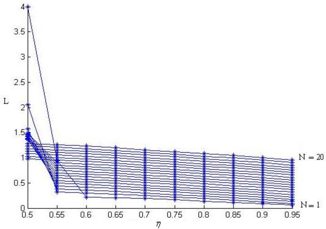
Figure 13. The length of uniform region based on number of heat sources and temperature uniformity coefficient
