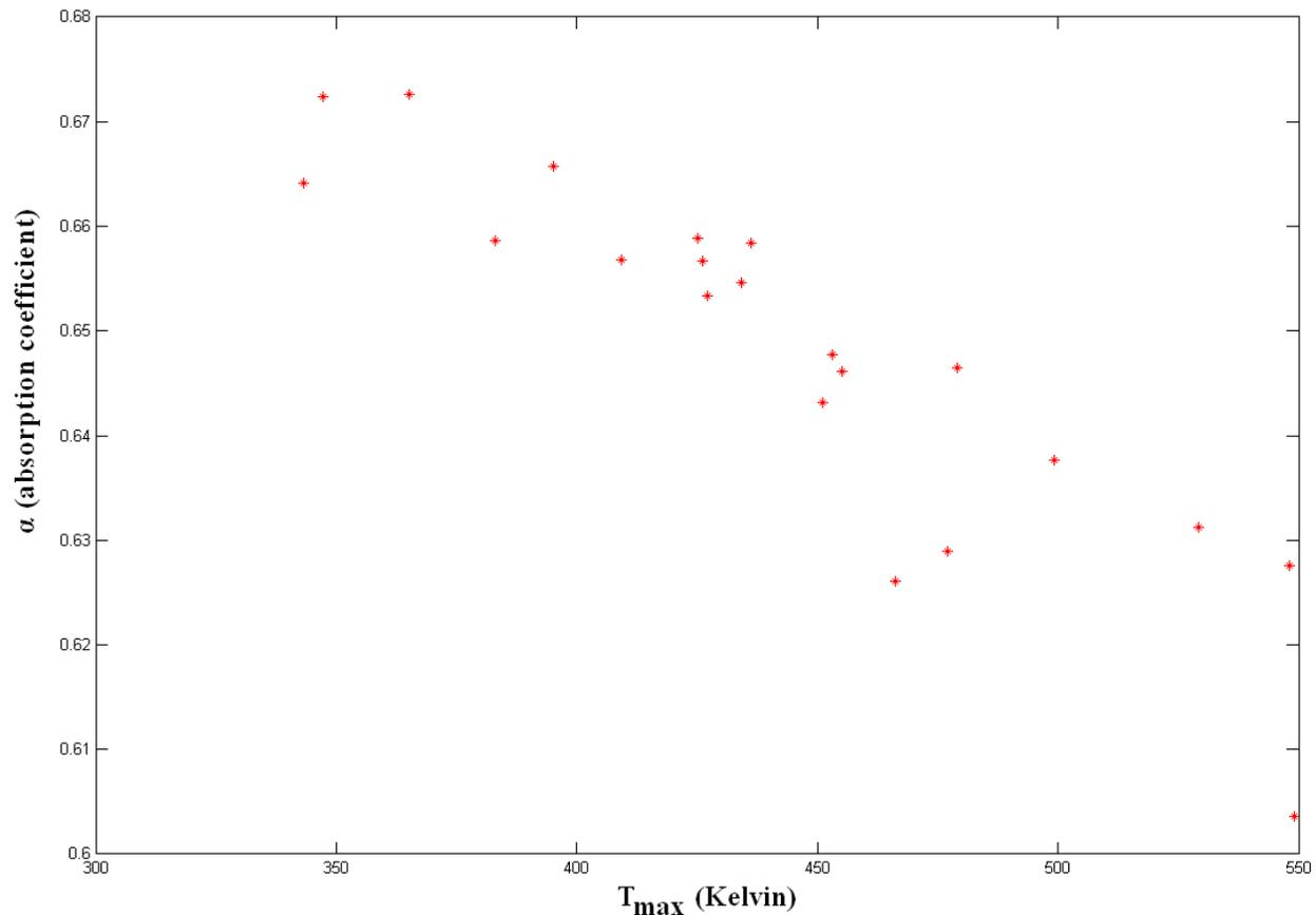
Figure 6. Relative absorption coefficient of unpainted steel and black painted as a function of Temperature
