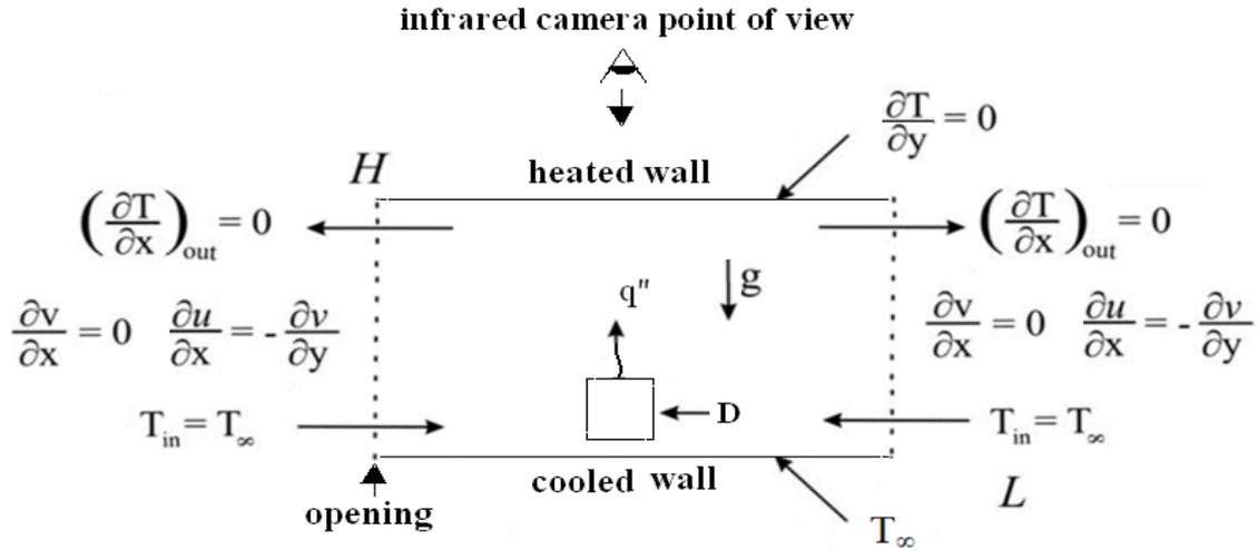
Figure 7. Schematic of the enclosure with discrete heaters, the coordinate system and boundary conditions
