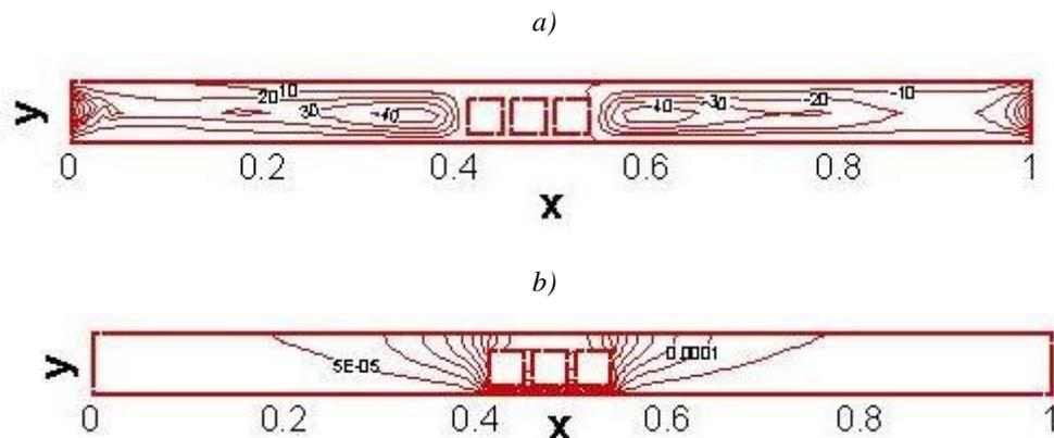
Figure 10. Dimensionless a) Streamline b) isotherm of three lamps ( $P_1=417$  W,  $P_2=298$  W,  $P_3=366$  W,  $H=3.5$  cm)
