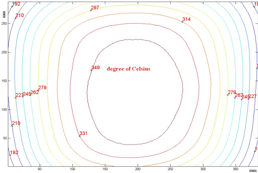
Figure 4. Contour of temperature on the heated plate
