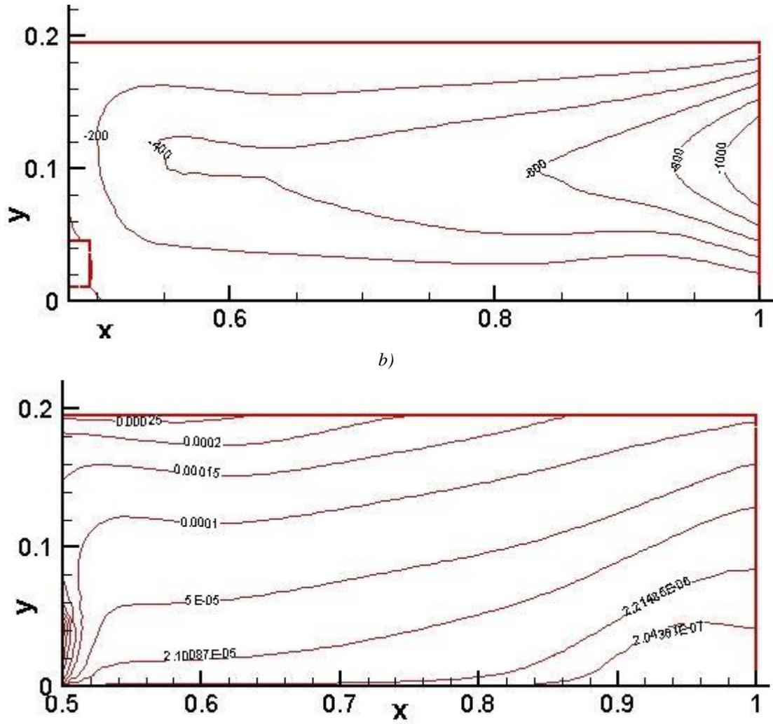
Figure 8. Dimensionless a) Streamline b) isotherm of one lamp (Q=1770 W,H= 19.5 cm)
