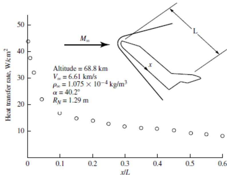
Figure 1. Required heating of a sample shuttle as a function of its distance from nose.
