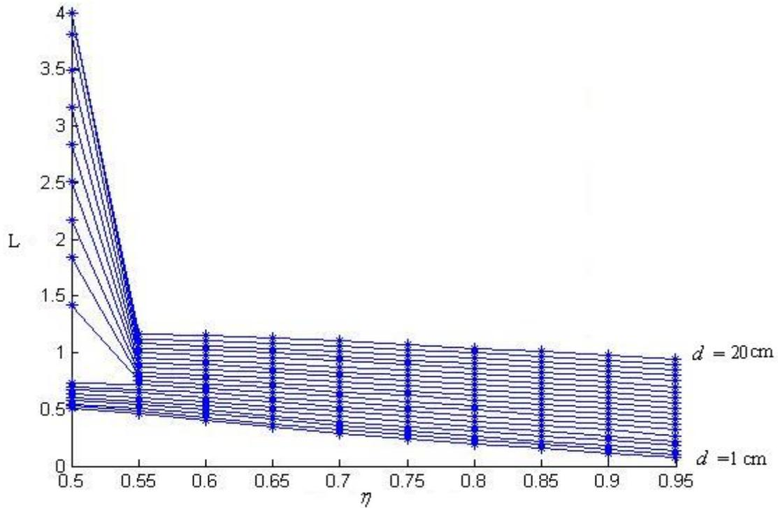
Figure 12. The length of uniform region based on distance between lamps and temperature uniformity coefficient
