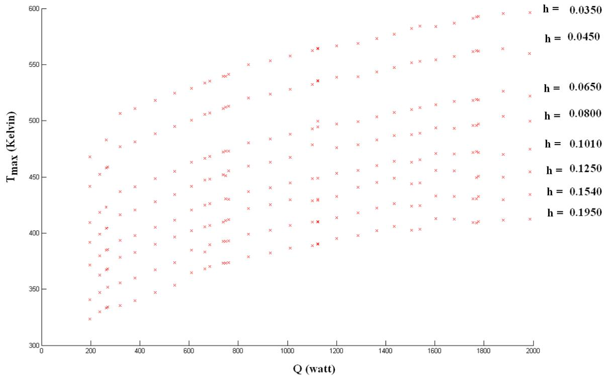
Figure 5. Maximum Temperature of the heated plate as a function of heat source power for various height of the plate
