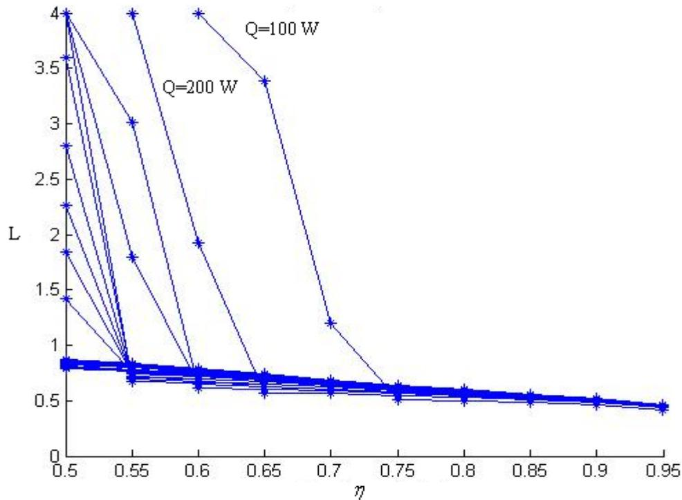
Figure 11. The length of uniform region based on power of lamps and temperature uniformity coefficient (d=10 cm,H=10 cm,N=10)
