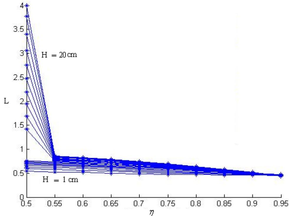
Figure 14. The length of uniform region based on Height of Plate from the Rack of Lamps and temperature uniformity coefficient ( $d=10$  cm, $N=10$ , $Q=1000$  W)
