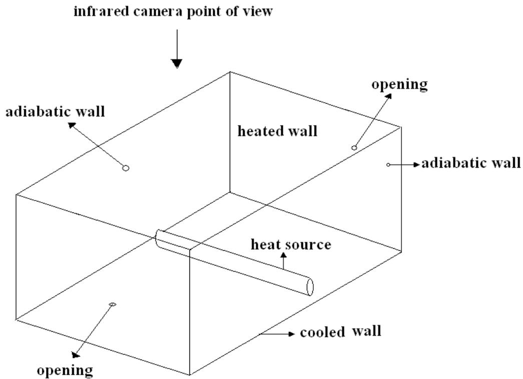
Figure 2. Schematic of the experiment: enclosure with discrete heaters and boundary conditions.
