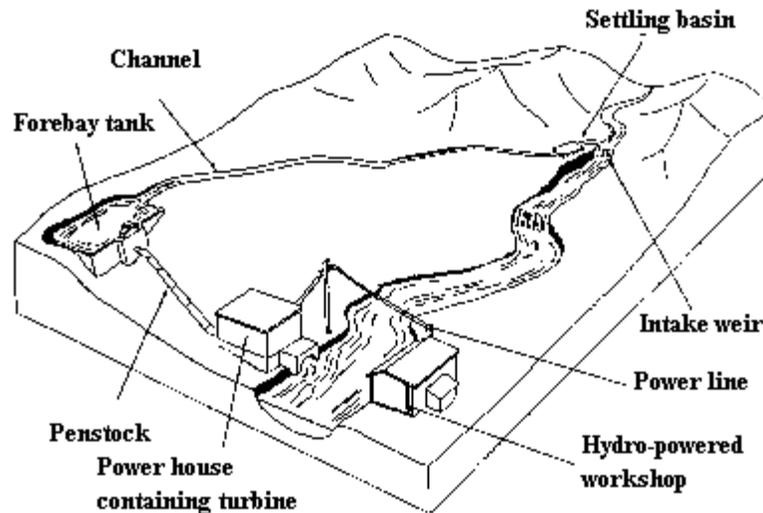
Figure 2: Layout of a typical micro hydro scheme [16]
