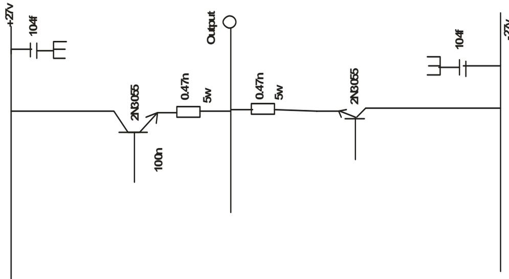
Figure 5 The output stage of power amplifier.
