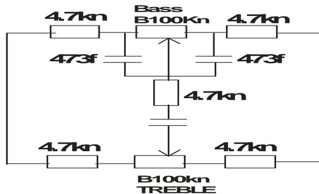
Fig 1 Independent Tone Control of Pre-amplifier circuit
