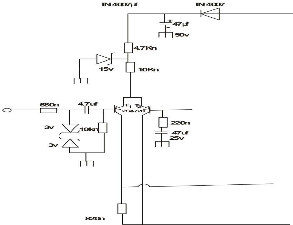
Fig 2 Input stage of power amplifier
