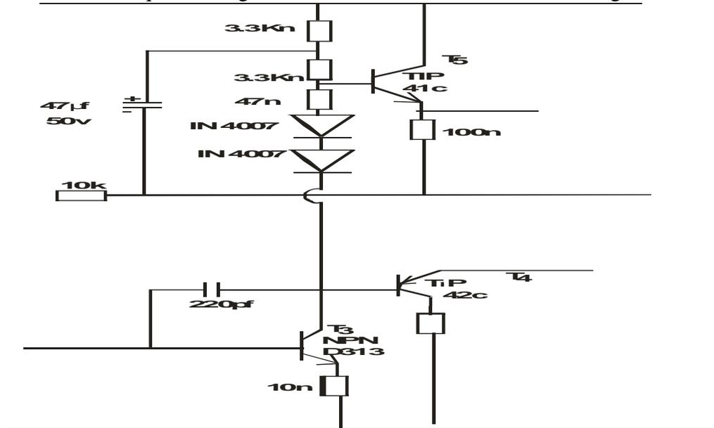
Figure 3 The amplification stage of power amplifier
