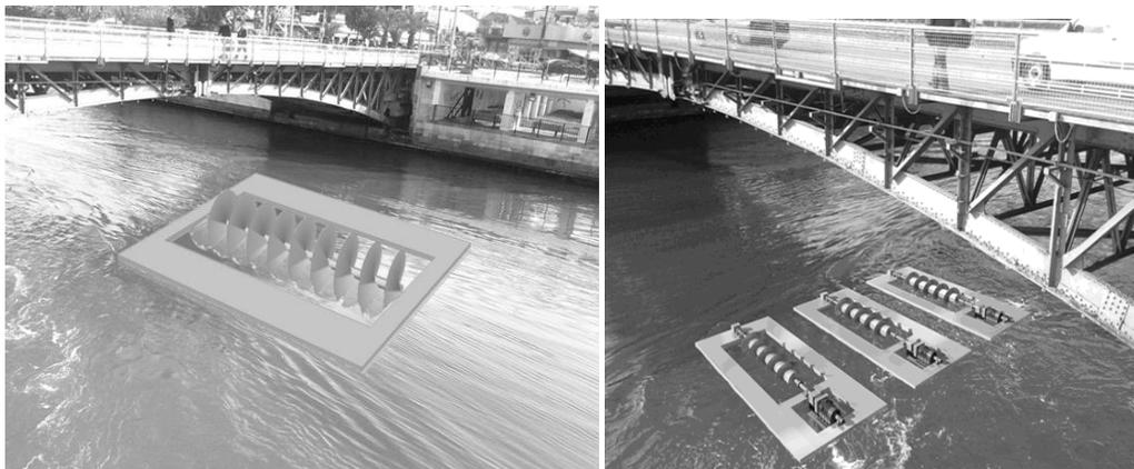
Figure 14. Photorealistic views of horizontal Archimedean rotor in Euripus Strait.
