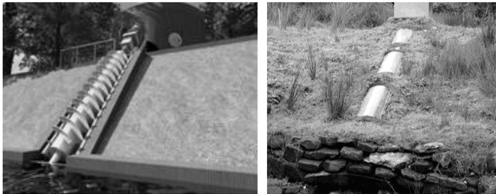
Figure 10. No tubular and tubular screw turbines applications
