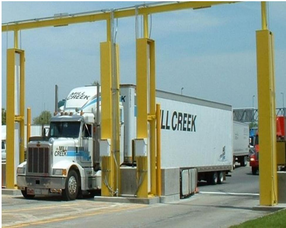
*Figure 1. Example screening location with four detector panels surrounding the vehicle.*
