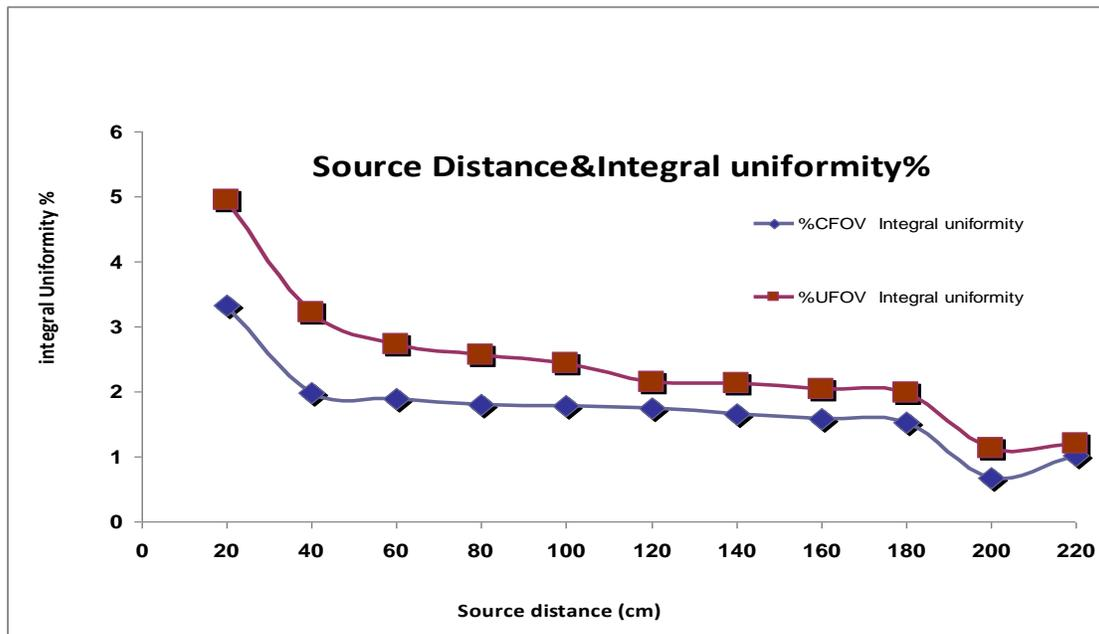
**Figure (1) : The integral uniformity versus source to detector distance**
