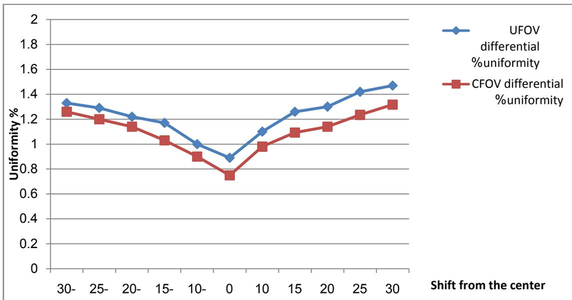
Figure (4): The differential uniformity versus the shift from the center.
