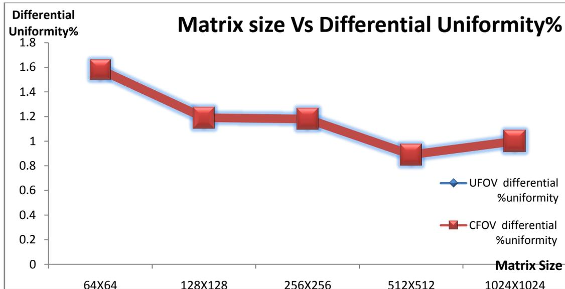
Figure (10): The differential uniformity versus the matrix size.
