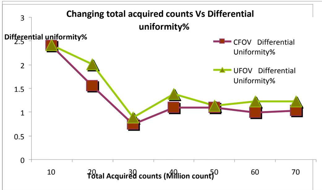
Figure (6): The differential uniformity versus the number of acquired counts.
