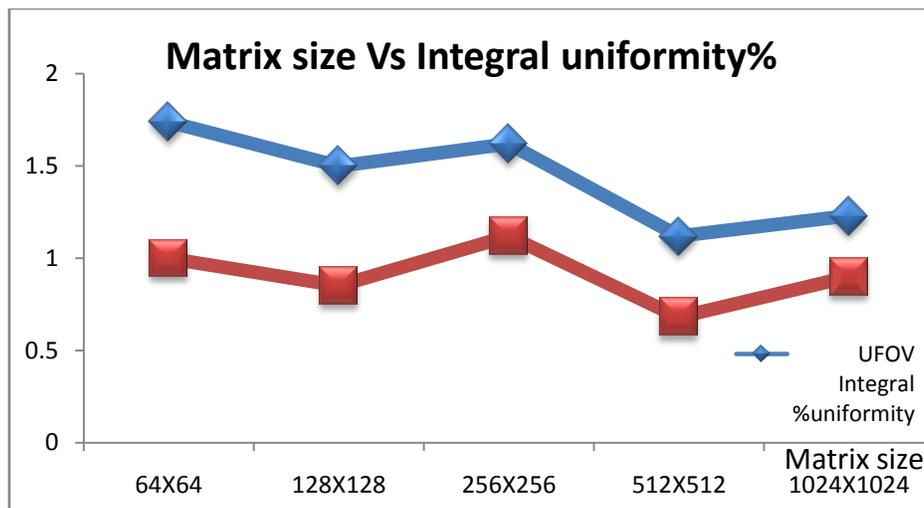
**Figure (9): The integral uniformity versus the matrix size.**
