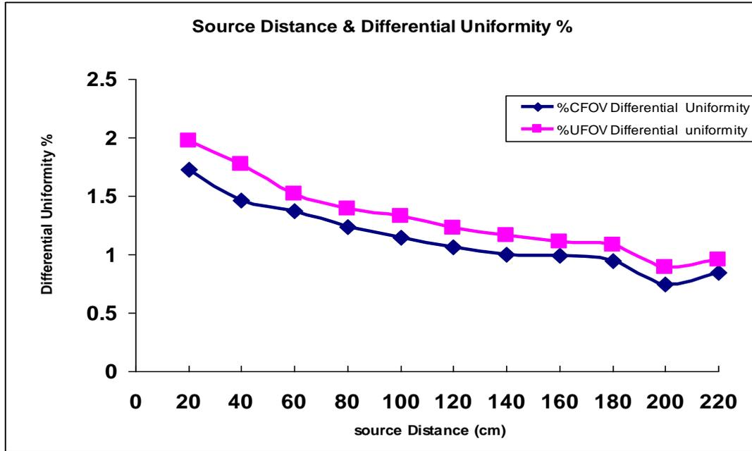
Figure (2): The differential uniformity versus source to camera distance
