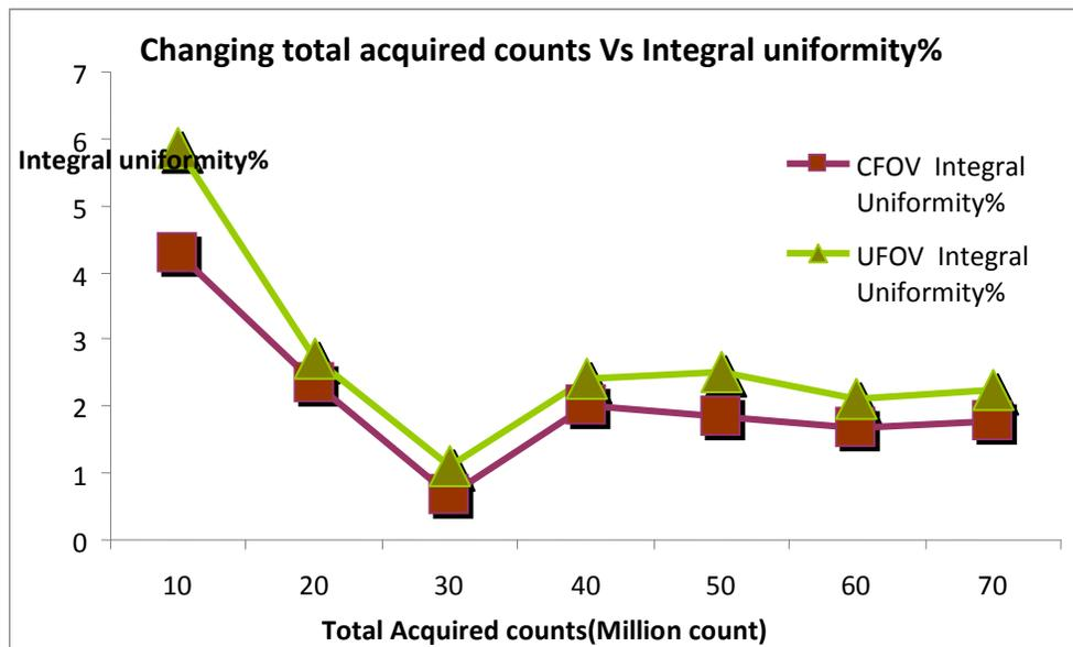
**Figure (5): The integral uniformity versus the number of acquired counts.**
