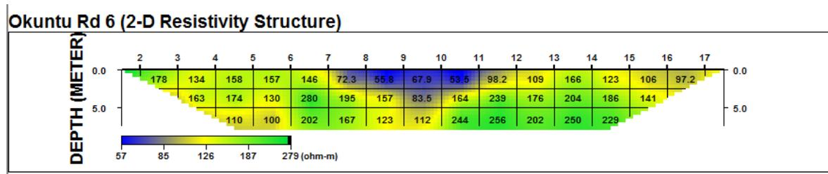
Figure 3f: Inverted 2D Resistivity structure along Dipole-Dipole profile (DP5) in Okuntu Road
