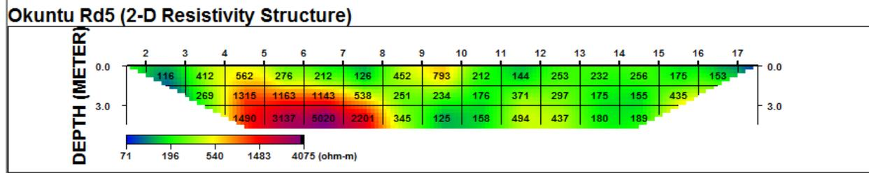
Figure 3e: Inverted 2D Resistivity structure along Dipole-Dipole profile (DP4) in Okuntu Road
