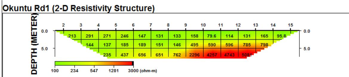
Figure 3a: Inverted 2D Resistivity structure along Dipole-Dipole profile (DP1) in Okuntu Road
