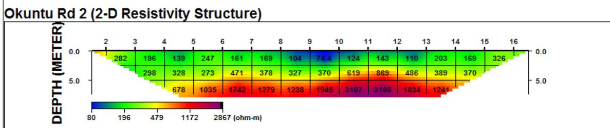
Figure 3b: Inverted 2D Resistivity structure along Dipole-Dipole profile (DP2) in Okuntu Road
