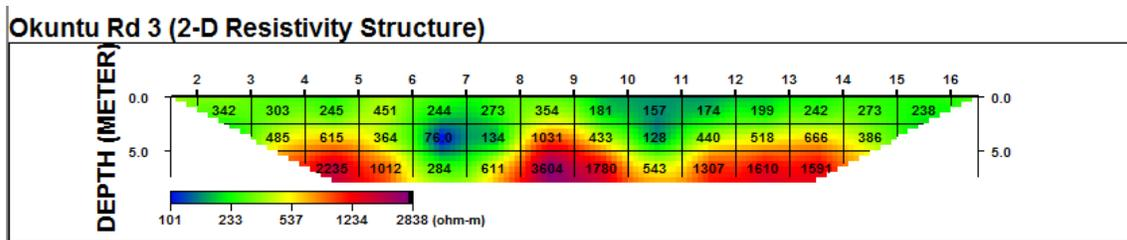
Figure 3c: Inverted 2D Resistivity structure along Dipole-Dipole profile (DP3) in Okuntu Road
