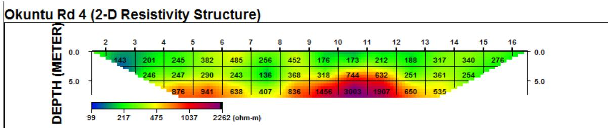
Figure 3d: Inverted 2D Resistivity structure along Dipole-Dipole profile (DP4) in Okuntu Road
