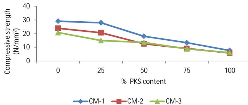
Figure 3. Compressive strength vs. % PKS content under different curing media for aggregate size of 5-20 mm.
